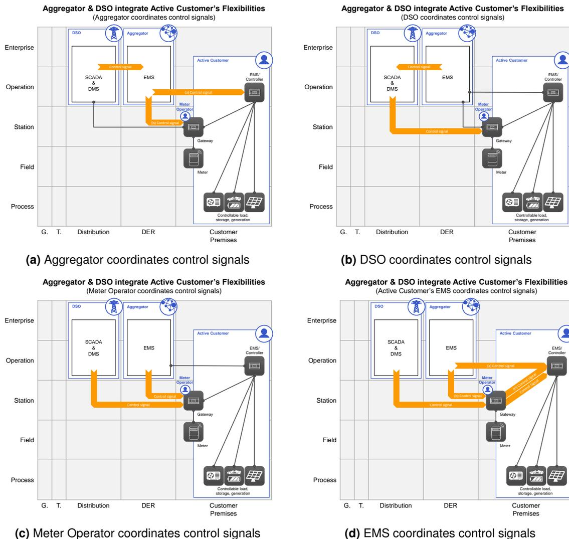
**Figure 7:** Four coordination approaches on how aggregator and DSO can integrate and coordinate the active customer's flexibility provision. The most relevant control signals are highlighted in orange. Grey connections are necessary to control, monitor or maintain the flexibility but are not in the foreground for the coordination. For simplicity, the meter operator is visualised purely as a role without the corresponding systems that are necessary for the meter operation.
